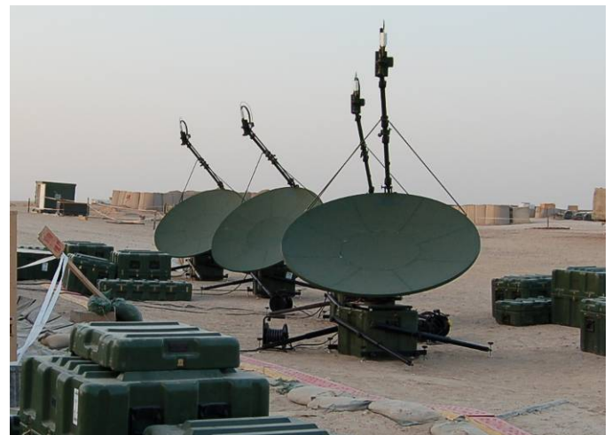
The DataPath V-SNAP Fly-Away is a compact yet powerful earth terminal specifically configured to interface with existing JNN and DKET networks.
