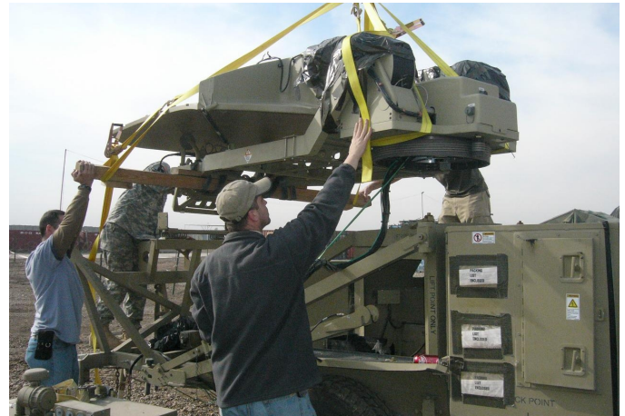
DataPath Field Engineers working with soldiers from the U.S. Army's 2 nd Brigade, 2 nd Infantry Division to repair a Satellite Transportable Terminal (STT) that was damaged in a direct mortar hit in Iraq in 2006.
